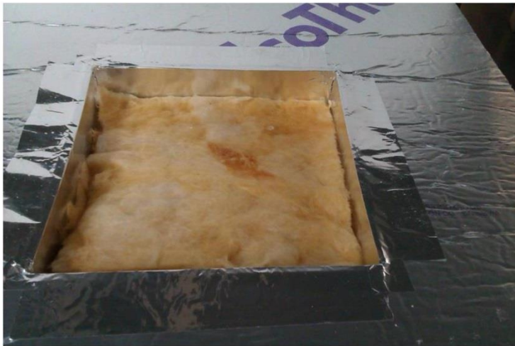
Figure 1. Glasswool inside the test chamber
