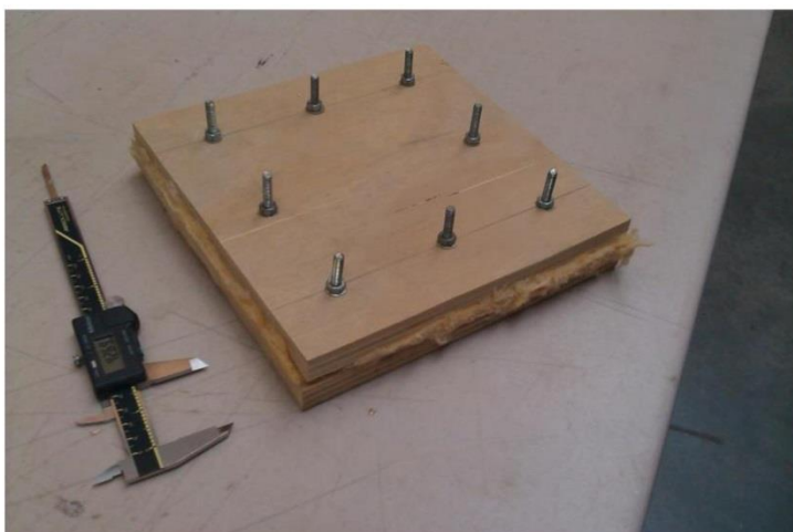
Figure 2. Glasswool in the compression plates, ready for testing
